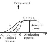
Changes in v causes changes in the maximum energy of the emitted photoelectrons and hence a change in the stopping potential.
