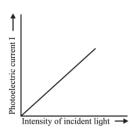
Collector at suitable +ve potential Frequency constant and above vo Intensity of light varied Current increases linearly with increase in Intensity Number of photoelectrons emitted per
